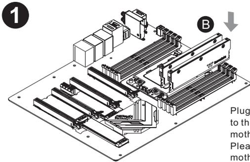
**1** Plug the Memory Module(B) to the DDR4 slot on the motherboard. Please refer to the motherboard manual for the installation location.
