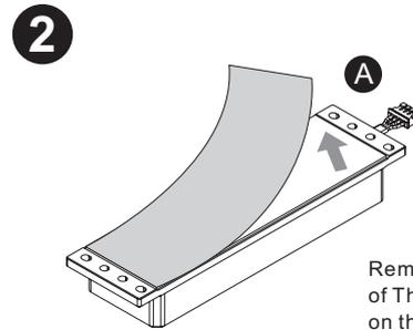
**2** Remove the protective film of Thermal Pad on the Water Block(A).
