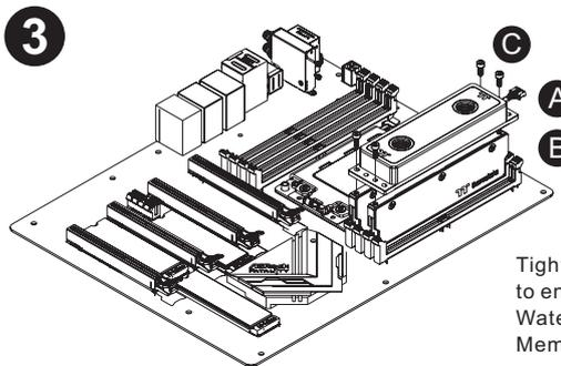
**3** Tighten the Screws(G) to enclose the Water Block(A) and Memory Module(B).
